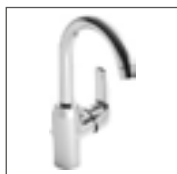
HANSAPINTO one-hole single-lever basin mixer, DN 15 4509 2283 chrome without pop-up waste, connection with flexible pressure hoses, HANSA 3S-Installation projection: 148 mm
