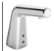
HANSADESIGNO STYLE electronic basin faucet, DN 15 battery-operated 5193 2201 chrome sensory operation (infrared), Mikado® Aerator, without pop-up waste projection: 100 mm
