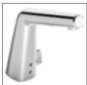
HANSADESIGNO STYLE electronic basin faucet, DN 15 battery-operated 5179 2201 chrome sensory operation (infrared), push-pop-up waste, flexible hoses projection: 138 mm
