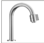
HANSANOVA basin pillar valve, DN 15 0091 8101 chrome for cold or pre-tempered water only projection: 127 mm
