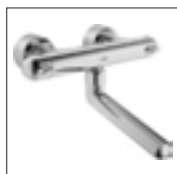
HANSACARE thermostatic shower faucet, DN 15 0830 2201 chrome safety stop against scalding at 38°C, eccentric connections with shut-off valve projection: 259 mm
