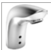
HANSAELECTRA electronic basin faucet, DN 15 battery-operated 6440 2211 chrome sensoryo peration (infrared), for cold or pre-tempered water only, without pop-up waste, hygienic flush after 72 h for 30 sec at factory preset projection: 96 mm
