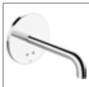
HANSAELECTRA trim kit with function unit concealed electronic mixer, DN 15 (G1/2) for cold or pre-tempered water only suitable for HANSABUEBOX concealed unit* 8180 2110 chrome projection: 245 mm
