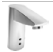
HANSAELECTRA electronicb asinfa ucet, DN 15 battery-operated 6491 2211 chrome sensoryo peration(inf rared), without pop-up waste, hygienic flush after 72 h for 30 sec at factory preset projection: 115 mm
