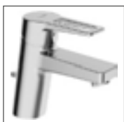
HANSATWIST one-hole single-lever basin mixer, DN 15 0909 2285 chrome loop lever (metal), pop-up waste (metal), connection with flexible pressure hoses projection: 121 mm
