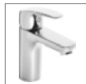
HANSAPINTO XL one-hole single-lever basin mixer, DN 15 4506 2283 chrome without pop-up waste, connection with flexible pressure hoses, HANSA 3S-Installation projection: 107 mm
