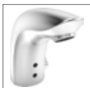
HANSAELECTRA electronic asinfa ucet, DN 15 battery-operated 6441 2211 chrome sensoryo peration(inf rared), without pop-up waste, hygienic flush after 72 h for 30 sec at factory preset projection: 96 mm
