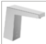
HANSALOFT electronic basin faucet, DN 15 mains supply 5748 2201 chrome sensor operation (infrared), incl. power supply and connection cable, push-pop-up waste projection: 143 mm
