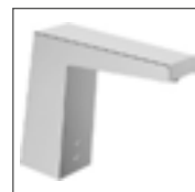
HANSALOFT electronic basin faucet, DN 15 mains supply 5748 2201 chrome sensory operation (infrared), incl. power supply and connection cable, push-pop-up waste projection: 143 mm
