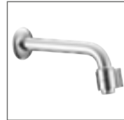
HANSANOVA wall-mounted basin valve, DN 15 0096 8101 chrome for cold or pre-tempered water only, can be shortened from 186 to 126 mm projection: 186 mm
