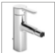
HANSADESIGNO STYLE one-hole single-lever mixer, DN 15 5173 3283 chrome for bidet, pop-up waste (metal), connection with flexible pressure hoses projection: 117 mm
